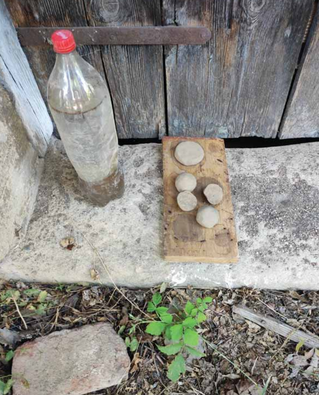
Testing the earth: bottle test, "cookies" and balls made of earth.
